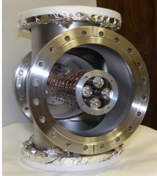
FIG. 1. The 30 cm long DC-drag cooling RFQ assembly.
